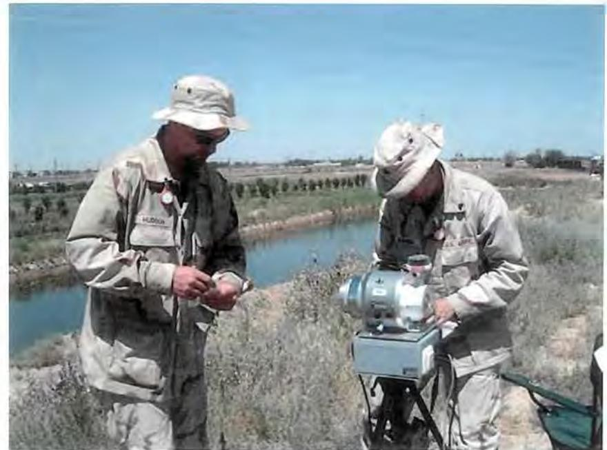
Figure D-5 (U): Air sampling for radioactive material
