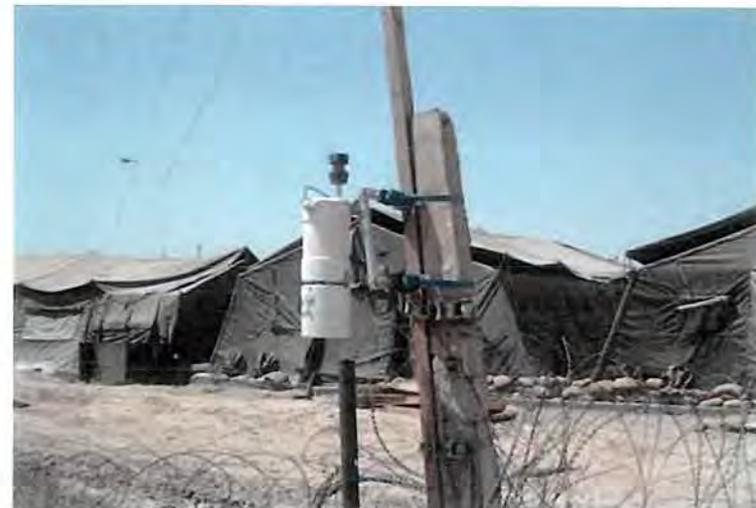
Figure D-22 (U): Ambient Air Monitoring with MiniVol in SSA Area
