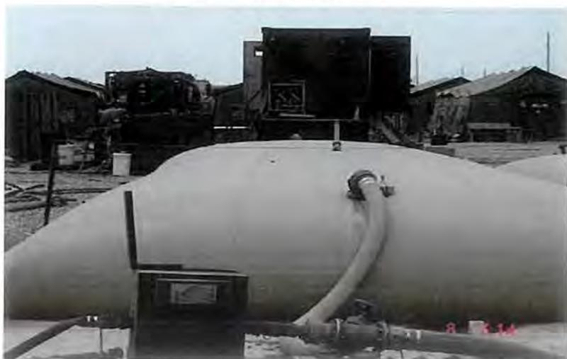
Figure D-17 (U): ROWPU Water Bladder
