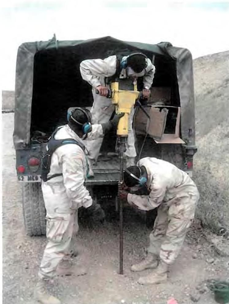
Figure D-13 (U): Subsurface Soil Sampling Using Bosch Hammer in Tent City Area
